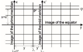
The graticule (metagraticule) has generally two axes of reflection symmetry. The horizontal one usually coincides with the axis y which is mostly the image of the equator.
