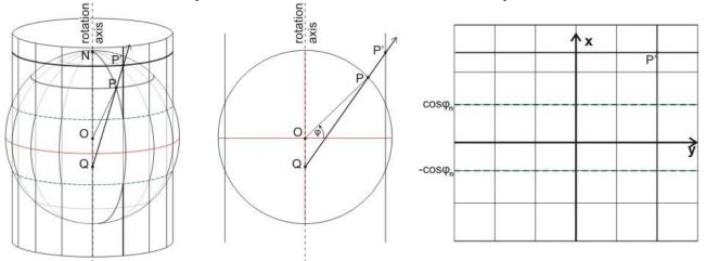
After cutting the superficies by one of its generators and unfolding it into a plane, the image of the graticule passes over a planar rectangular grid: a) the images of the parallels are **parallel straight lines**, b) the images of the meridians are **parallel straight lines**, too, c) they are **perpendicular** to each other, and d) the distance between the mapped meridians is **proportional** to the correspondent **longitude difference**.
