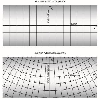
The grayscale level indicates the magnitude of the map distortions in the normal and oblique cylindrical projections (white shows negligible distortions)
