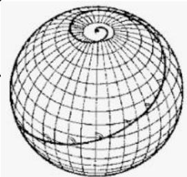
The coordinates  $\varphi$  and  $\lambda$  of the point P on the loxodrome arc will be changed by  $\Delta \varphi$  and  $\Delta \lambda$ . This establishes a small figure which is almost a small planar right triangle with the loxodrome arc  $\Delta s$  ("hypotenuse") as well as parallel arc R\*cos $\varphi$ \*arc $\Delta \lambda$  ("leg") and meridian arc R\*arc $\Delta \varphi$  ("leg").
