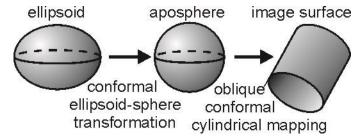
transformation and an oblique conformal cylindrical projection from the intermediate sphere to the plane).
